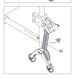
• Once the wheels are fitted, you can return the anti-tippers to their starting position. To do this, push the wheelchair forwards and push back the holding rod [95] using your foot at the same time.
