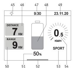
When the control unit is switched on, the Alber start screen (if activated) appears first and, after about 3 seconds, this changes to the user screen illustrated in the adjacent diagram. The diagram shows all the symbols that can be shown on the control unit display.
