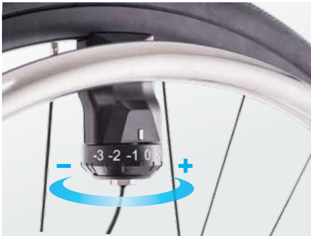
Sensitivity of the push rim sensors adjustable in seven increments
