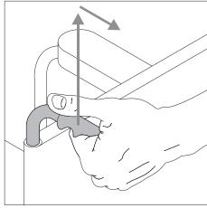
• Whilst doing so, pull the wheelchair by its handles a little upwards and to the rear until the wheelchair has been raised and the anti-tippers click into a fixed position.
