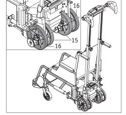
To take the wheelchair drive wheels with you across the stairs, use the wheel transport bracket available as an accessory for your scalamobil. This bracket is only of use, if there is sufficient space on the stairwell. This means that the wheelchair wheels do not need to be carried separately.
